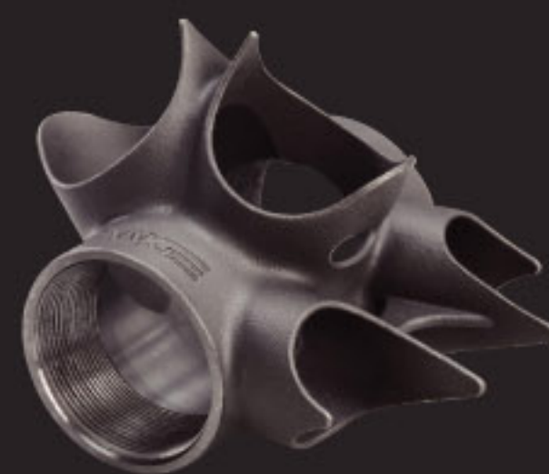
Model: TB003 B.B Shell Tube: 34.9*31.8*22.2mm Angle: 60°*64°*7° W.T.: 160g
