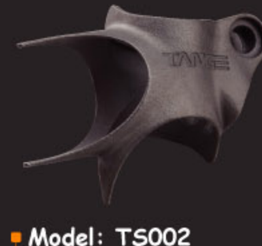
Model: TS002 Seat Lug Tube: 31.8*31.8mm Angle: 73°, 30° For 26.6mm Seat Post Seat Pin dia.: 8.2mm Seat Stay: any angle Seat Stay tube: 10.6*13.2 W.T.: 60g
